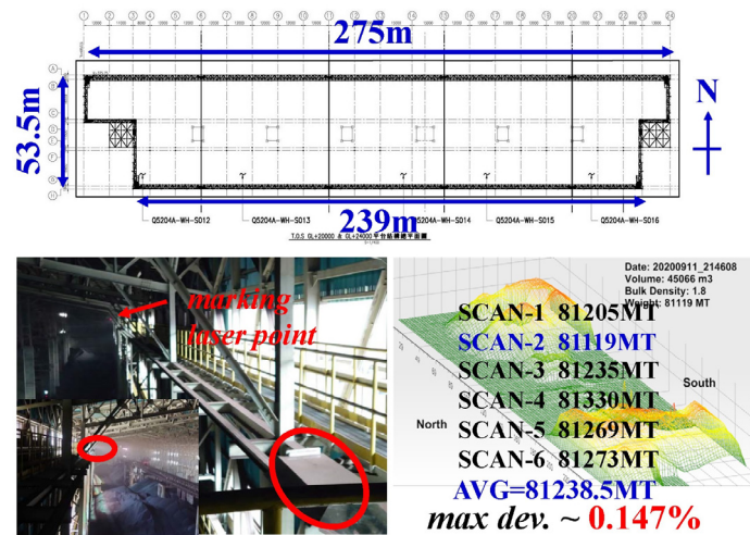
Fig.16. Arrangement and measuring results of the indoor rail-guided vehicle
